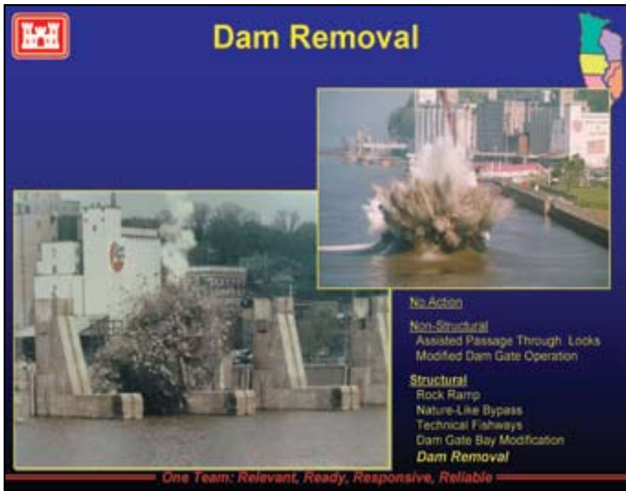
Army Corps slide shows a structural option to facilitate fish passage. (From link on website of Jim Bensman)
