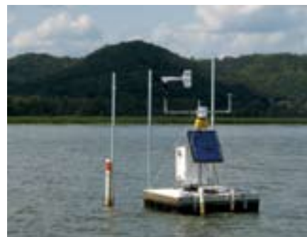
Pool 8 monitoring equipment includes round yellow buoys near the Main Channel that measure dissolved oxygen (top), and dock platforms in backwater areas that measure oxygen, water clarity, wind, light and water depth. (courtesy of U.S. Geological Service)
